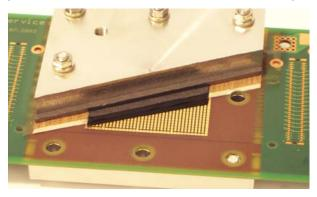
The gas diffusion layer will be placed directly on the segments. The channels of the flow field are milled between the segments. The device is usable as anode or cathode of a single cell.
